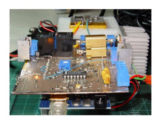
MOSFET R<sub>DS(on)</sub> Tester PCB has four ground planes
